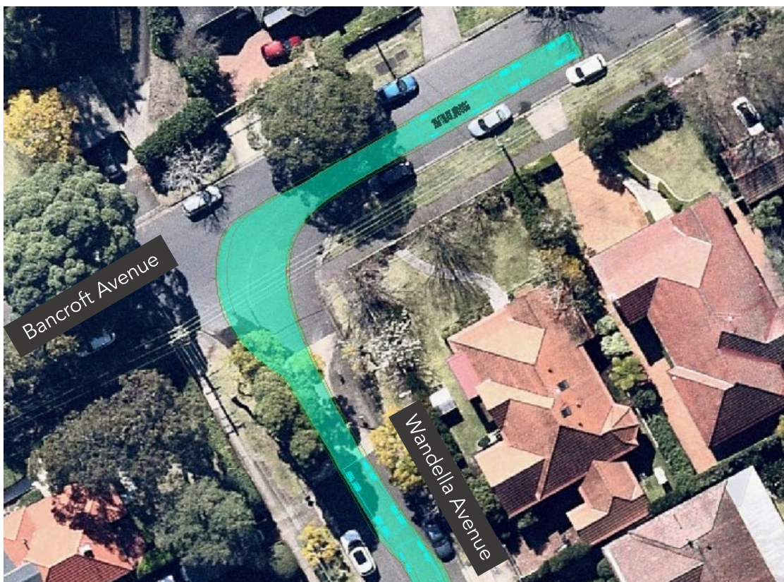
Figure 4-6: 19m Truck and Dog at intersection 3 (Bancroft Avenue/Wandella Avenue)
