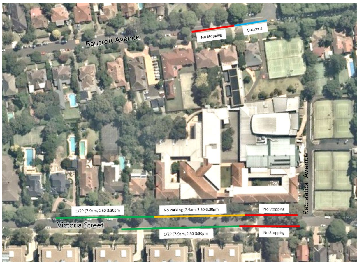
Figure 3-2: Existing On-Street Parking Controls
